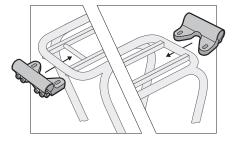
2. Place one clamp on each end of the rack (front and rear). Insert clamps from below and line up with the two fittings on the underside of the rack.
