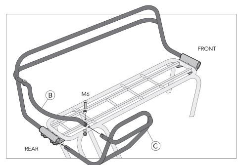
5. Insert lower end of right rail (C) from the right side into the center of the clamp until it comes to a stop while connecting the upper end to the rear rail (B) as shown.
