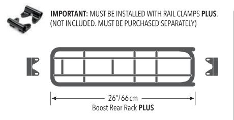
**IMPORTANT:** Notes to mechanic: See Instructions. Install Benno rail clamps and rails only on compatible Benno rear racks and use only pre-drilled holes and fittings. Do not mount clamps and rails to damaged racks. Use only original Benno rails with the Benno rail clamps. Do not modify clamps, racks or rails, change position or drill new holes as this will void any warranties and/or claims for liability.
