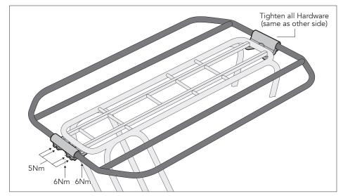
6. Once all pieces are installed, adjust and straighten rails and clamps as needed.
