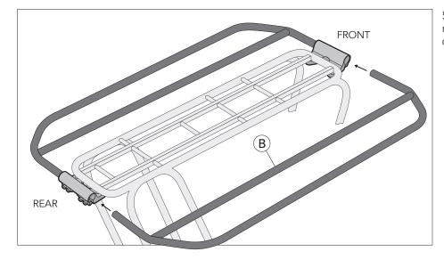
5. Insert both ends of rail (B) from the right side all the way into the center of the clamps until they come to a stop.
