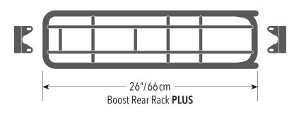
**IMPORTANT:** *Notes to mechanic:* See diagram. Install Benno Rail Clamps PLUS and Rails PLUS only on compatible Benno Boost Rear Racks PLUS and use only pre-drilled holes and fittings. M5 bolts are to be tightened to 5Nm and M6 bolts to 6Nm. Do not mount clamps and rails to damaged racks. Use only original Benno Rails PLUS with Benno Rail Clamps PLUS. Do not modify clamps, racks or rails, change position or drill new holes as this will void any warranties and/or claims for liability.
