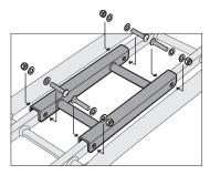
2. Insert included hardware as shown and tighten nuts to 4.9 Nm. DO NOT CHANGE POSITION OR MODIFY ADAPTER OR RACK.
