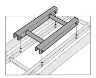
1. MUST BE INSTALLED BY MECHANIC AT AUTHORIZED BENNO DEALER. Line up Adapter with all four predrilled holes in Benno Rack and set in place.
