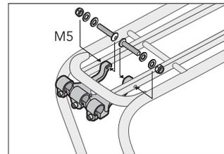
4. Insert smaller M5 bolts through clamp arms and pre-drilled holes in square center tubes. Place washers and self-locking nuts as shown. **TIGHTEN NUTS SLIGHTLY – CLAMP STILL NEEDS TO BE ABLE TO MOVE.**
