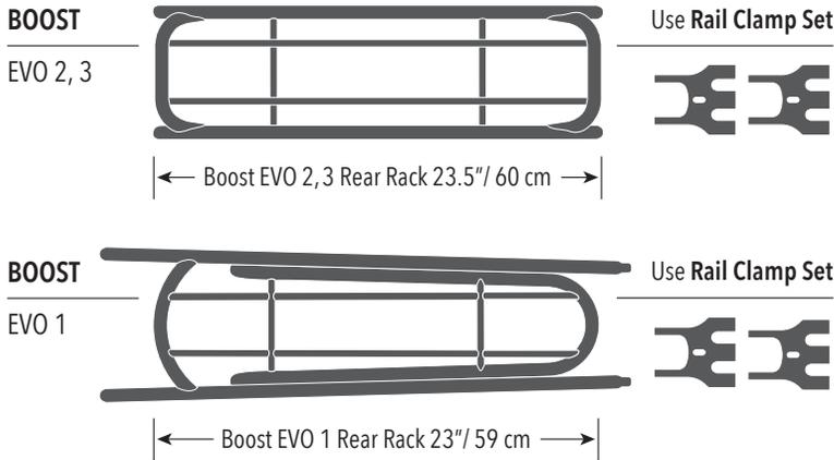
**IMPORTANT: Notes to mechanic:** See diagram. Install Benno Rail Clamps and Rails only on compatible Benno Boost Rear Racks and use only pre-drilled holes and fittings. M5 bolts are to be tightened to 5Nm and M6 bolts to 6Nm. Do not mount clamps and rails to damaged racks. Use only original Benno Rails with Benno Rail Clamps. Do not modify clamps, racks or rails, change position or drill new holes as this will void any warranties and/or claims for liability.
