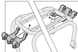
2. Place one clamp on each end of the Benno Utility Rear Rack (front and rear). Insert clamp from below, position between the square center tubes and line up with pre-drilled holes.
