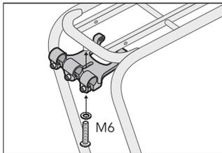
3. Insert large M6 bolt and washer through the slotted hole of the clamp and screw into the fitting on the underside of the rack. **TIGHTEN BOLT SLIGHTLY – CLAMP STILL NEEDS TO BE ABLE TO MOVE.**
