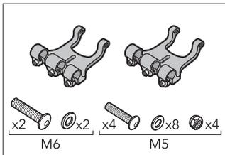
1. Ensure correct hardware count before installation. Separate the 2 larger M6 bolts and washers from the 4 smaller M5 bolts, washers and self-locking nuts.
