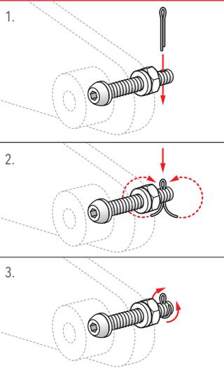
**IMPORTANT:** *Notes to mechanic:* See diagram. Install Trailer Adapter only on compatible Benno Boost E and use only pre-drilled holes and fittings. Do not mount to damaged bikes. Use only original hardware included. Do not modify adapter, mounting points on bike, change position or drill new holes as this will void any warranties and/or claims for liability. Ensure firm and proper installation and function.
