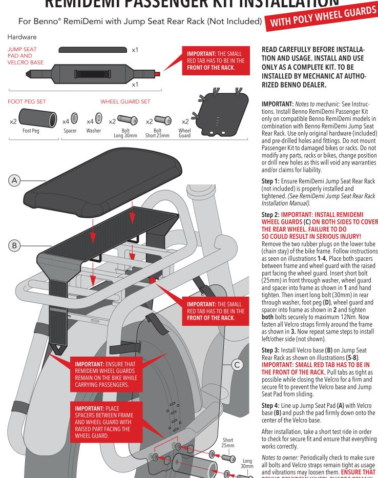
**READ CAREFULLY BEFORE INSTALLA-**TION AND USAGE. INSTALL AND USE ONLY AS A COMPLETE KIT. TO BE **INSTALLED BY MECHANIC AT AUTHO-**RIZED BENNO DEALER.
