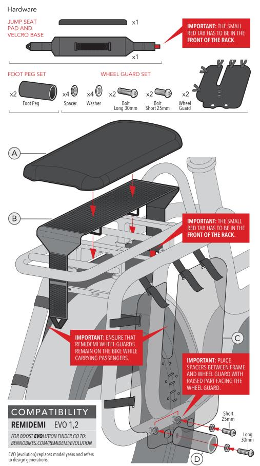
READ CAREFULLY BEFORE INSTALLA-TION AND USAGE. INSTALL AND USE ONLY AS A COMPLETE KIT. TO BE INSTALLED BY MECHANIC AT AUTHO-RIZED BENNO DEALER.
